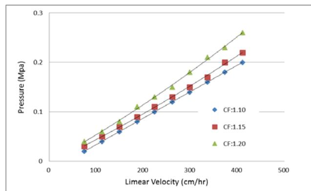
In this column format Cellufine A-500 showed good flow properties over a range of packing compression factors (Cf) from 1.10 to 1.20 while keeping the back pressure < 0.3MPa.
