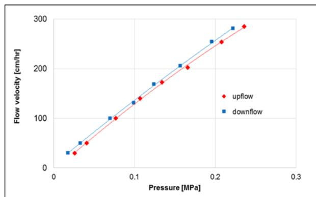
Column was packed from a 50 % slurry in water at 0.15 MPa for 30 min to a final bed height of 19.2 cm with a compression factor (Cf) of 1.20. The above data shows that a 45 cm ID column can be packed with Cellufine sulfate (particle size: 70 μm) at an optimal compression factor of 1.02 and operated at flow rates up 300 cm/h (7.9 L/min flow rate) under 0.3MPa back pressure in both flow directions.
